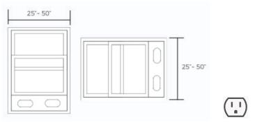
The window installation kit allows you to install the air conditioner in most vertical sliding windows  $25^{\prime\prime}$  to  $50^{\prime\prime}$  wide, or horizontal·s1iding windows from  $18^{\prime\prime}$  to  $50^{\prime\prime}$  high.
