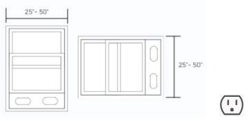
The window installation kit allows you to install the air conditioner in most vertical sliding windows 25" to 50" wide, or horizontal-s1iding windows from 18" to 50" high.
